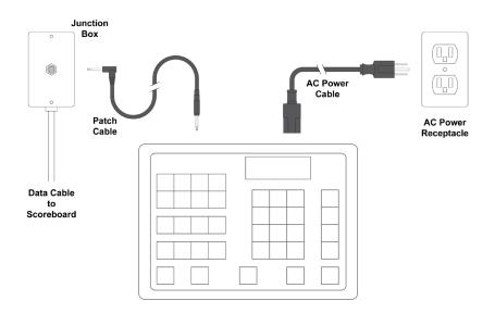
system, the power receptacle may be the only consideration on the console side of installation. For details about ScoreLink, consult the documentation that ships with the product. Otherwise use the stereo patch cable to plug the console into the junction box.
